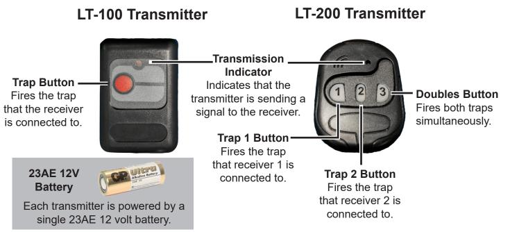
Your transmitters and receivers are preset to the required channel and trap ID to fire the designated trap(s). Simply press the trap button to fire the corresponding trap. The LT-200 has the added abilities to fire a second trap and a true pair. Press button 3 on the LT-200 transmitter to fire both traps simultaneously.
