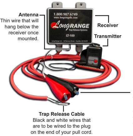
The LT-100 includes 1 receiver with a 1 button transmitter. The LT-200 includes 2 receivers with a 3 button transmitter. The 2 receivers included with the LT-200 will be labeled with Trap 1 and Trap 2. The receivers include 2 mounting holes and it is recommended that the receivers are mounted on a non-metal post, **2-3 feet high** with the antenna hanging below the receiver.
